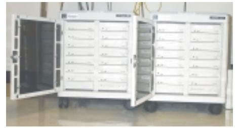
These Library Systems' CDROM towers can access 28 different CDROM-archived data bases, according to patrons' requests.
